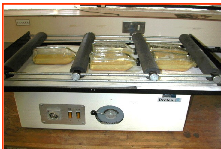
Figure 6.1: Fractionation of compounds by means of liquid-liquid extraction using a mechanical shaker.
