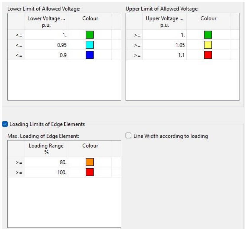
DIgSILENT software indicating the colour coding in the network
