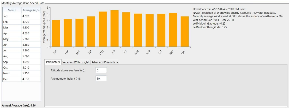
Figure 40 Monthly Average Wind Speed Data in Likhaebaneng river in the Quthing district
