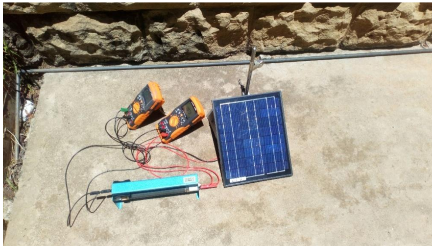
Figure 2; Experimental arrangement of testing solar panel
