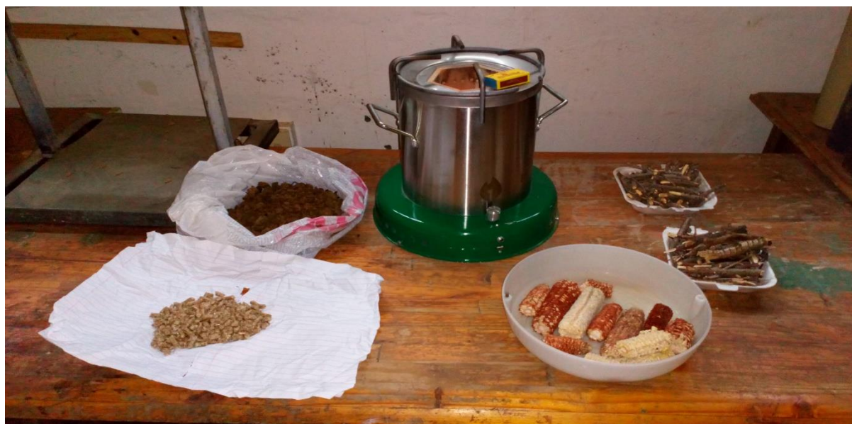
Figure 1; Biomass fuel cut into pieces that can fit into the chamber
