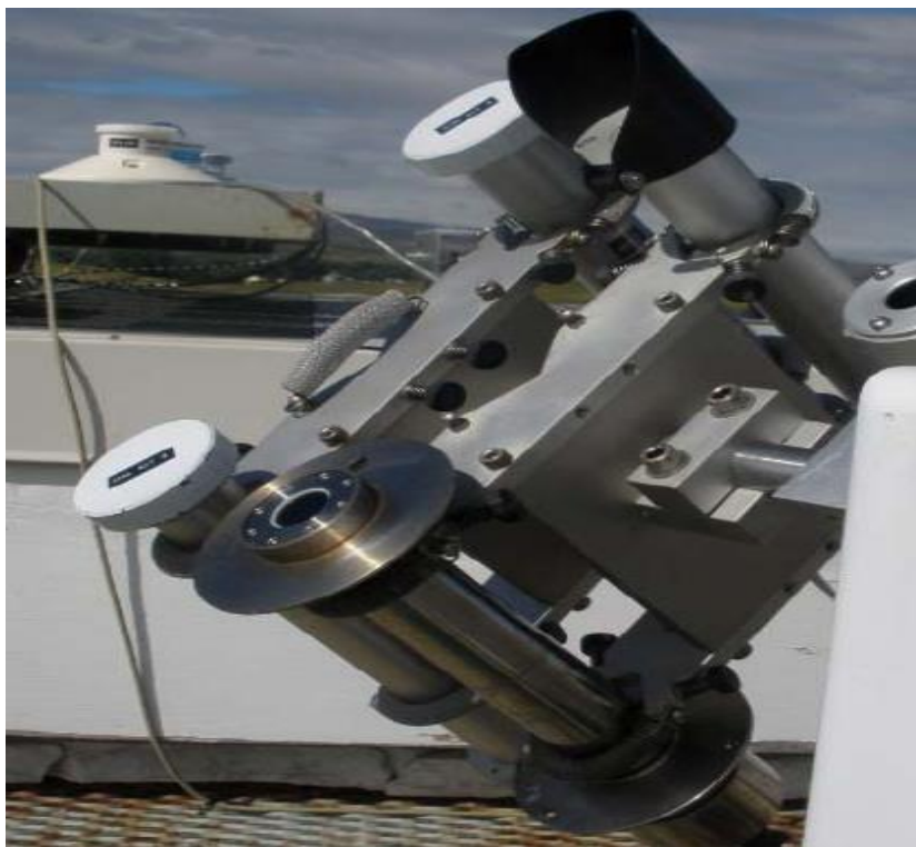
Fig 2.2. 1 A pyrheliometer instrument for measuring beam solar radiation. Source : The Australian Government, Bureau of Meteorology [53]
