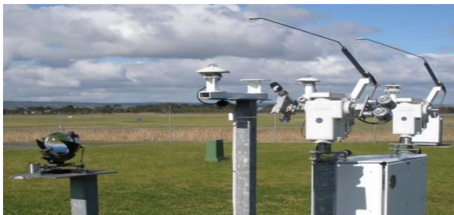
Fig 2.2. 7 A weather station with a typical solar radiation measuring equipment.
