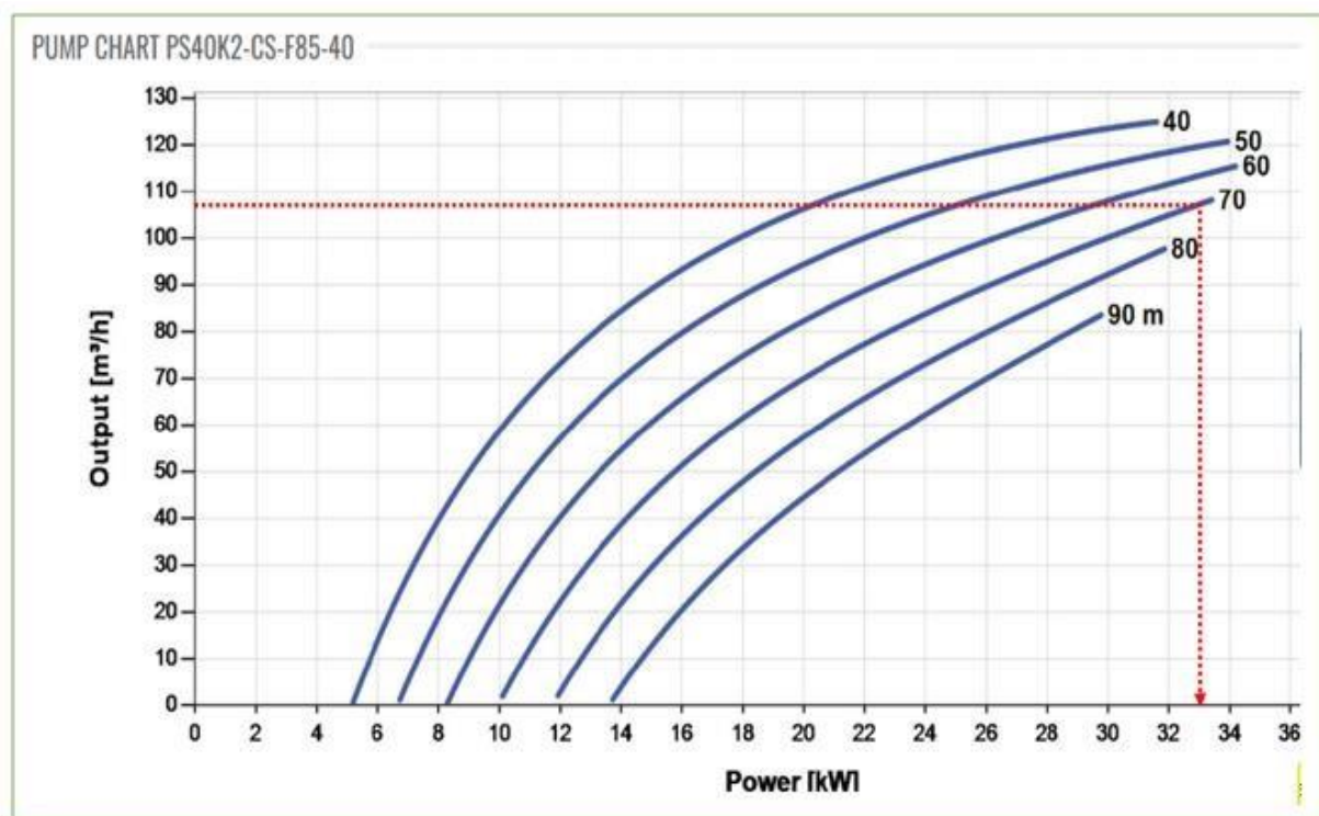
Figure 36: Selected pump (PS40K2-CS-F85-40) performance curve [93].
